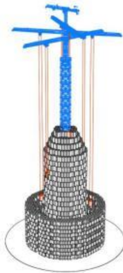
Figure. 1.2. Tower Solid Gravity Energy Storage Fyke, A. (2019)
