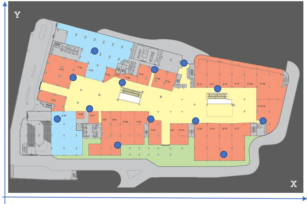
Figure 3.1 Example of sensor layout on mall floorplan
