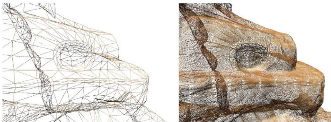
Figure 2.7 Comparison between geometry of original mesh (left) and result of applying tessellation shader (right)
