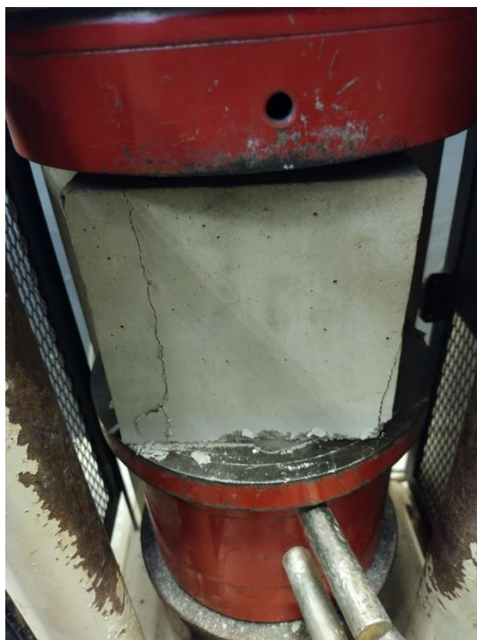
Figure 3.13: Cracking during Compression Test.
