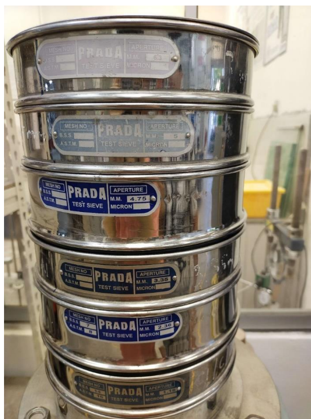
Figure 3.2: Setup of Sieves and Pan.
