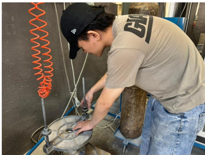
Figure 3.3: Setup of Sieving Machine.
