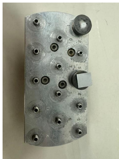
Figure 3.12: Sample Platform and Holder for SEM and EDS test.
