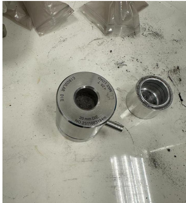
Figure 3.7: Stainless Steel Mould with 20mm Diameter.
