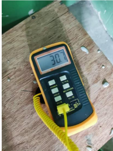
Figure 3.29: Measuring of Concrete Temperature.
