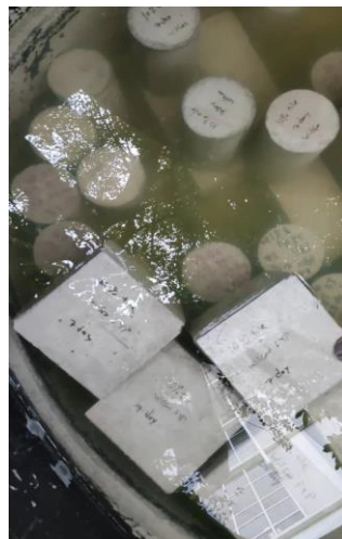
Figure 3.30: Curing of Concrete.
