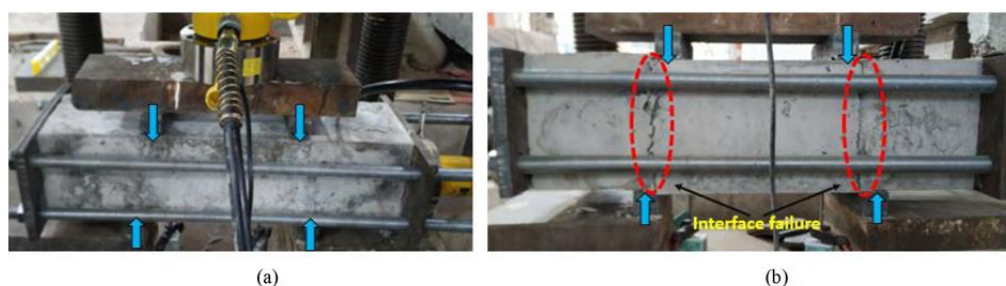
Figure 2.14: Failure Mode of Concrete Interface with Grooved Surface (Wu, Ayinde and Zhou, 2022).
