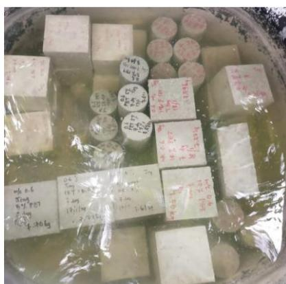
Figure 3.15: Water Curing.
