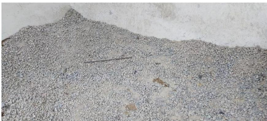
Figure 3.4: Limestone Gravels as Coarse Aggregates.
