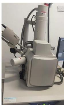
Figure 3.21: Hitachi S-3400N SEM Machine.
