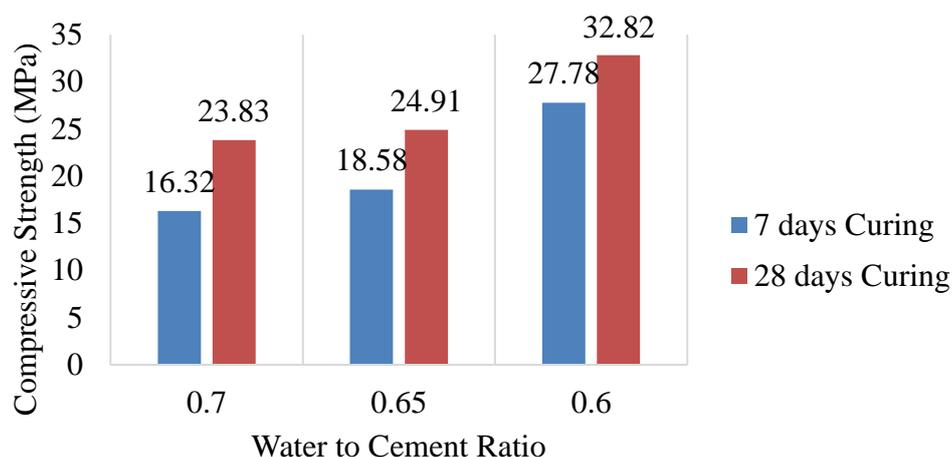
Figure 4.7: Compressive Strength (MPa) of Trial Mixes of PET-5.
