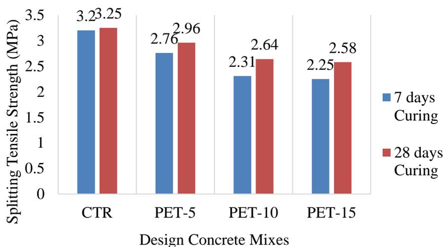
Figure 4.11: Splitting Tensile Strength of Various Design Concrete Mixes.
