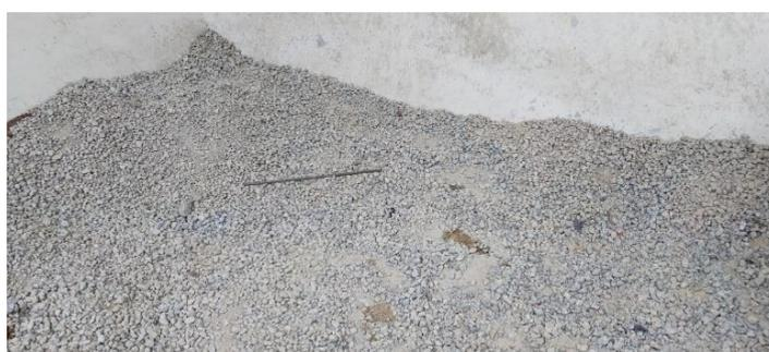
Figure 2.15: Limestone Gravels as Coarse Aggregates.
