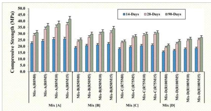
Figure 2.10: The Compressive Strength of Concrete with different Portion of Metakaolin used (Elhadi et al., 2023).
