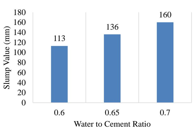
Figure 4.5: Slump Test of Trial Mix PET-5 with Various W/C Ratio.
