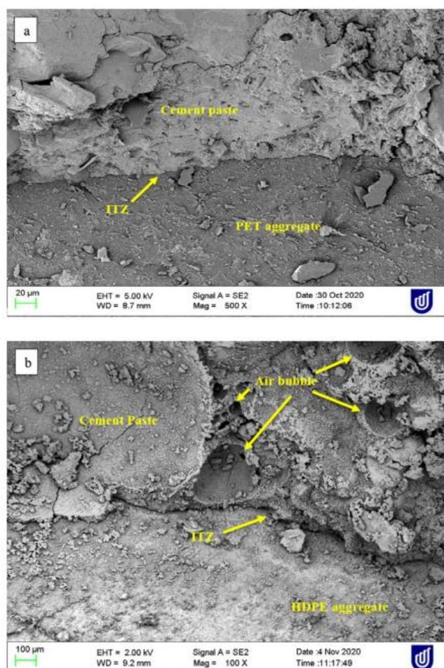
Figure 2.16: SEM Images of Concrete Mixture Containing Recycle Plastic Aggregates (Abu-Saleem et al., 2021).
