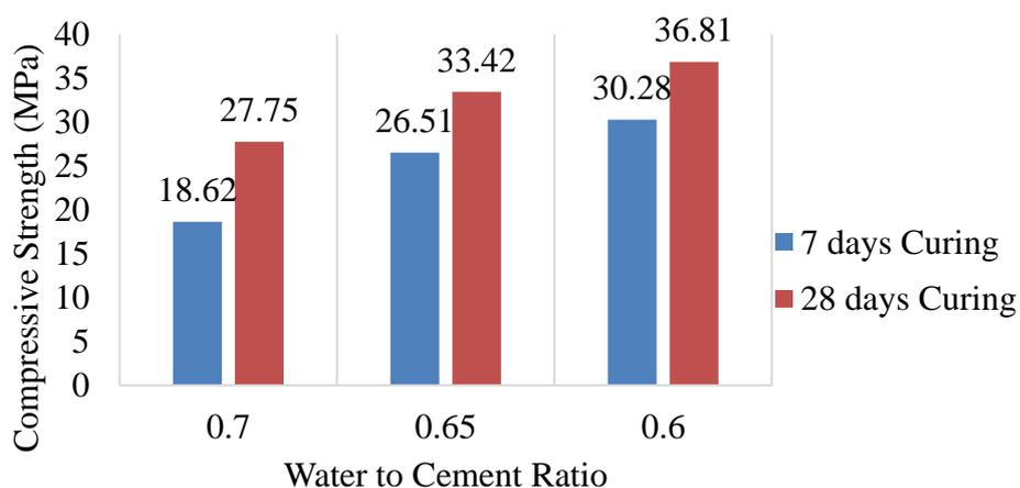
Figure 4.4: Compressive Strength (MPa) of Trial Mixes of CTR.
