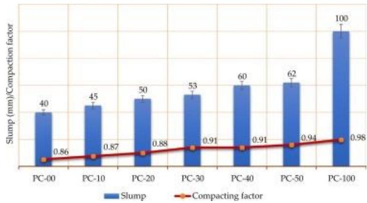
Figure 2.8: Slump and Compacting Factor Test of Fresh Concrete with various PET content (Bamigboye et al., 2022).
