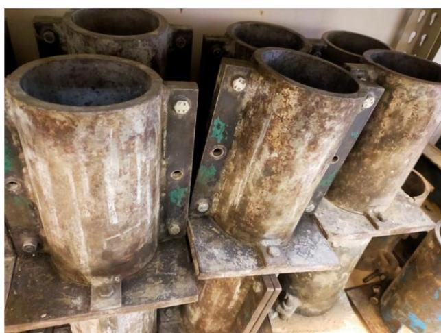
Figure 3.8: Cylindrical Mould.
