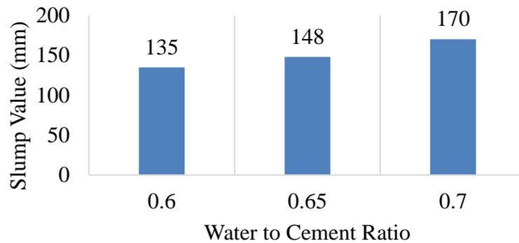
Figure 4.2: Slump Test of Trial Mix CTR with various W/C Ratio.
