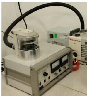
Figure 3.20: Emitech SC7620 Coater Machine.
