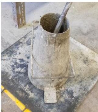
Figure 3.16: Slump Cone for Slump Test.
