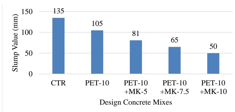
Figure 4.12: Slump Values of Various MK Content in PET-10.
