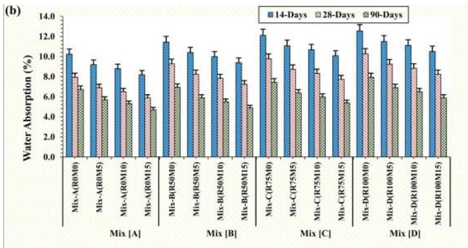
Figure 2.12: The Percentage of Water Absorption of Concrete with different Portion of Metakaolin used (Elhadi et al., 2023).
