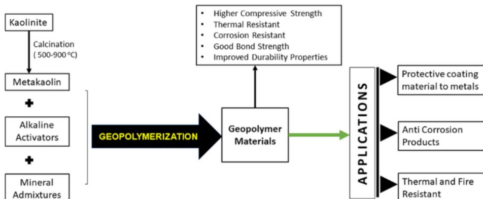
Figure 2.13: The Application of Metakaolin (Jindal et al., 2022).
