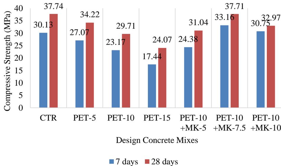
Figure 4.25: Summary of Compressive Strength of Design Concrete Mixes.
