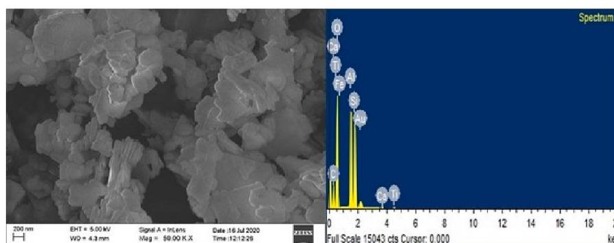
Figure 2.17: SEM and EDX Analysis of Metakaolin (Gopalakrishna and Pasla, 2023).
