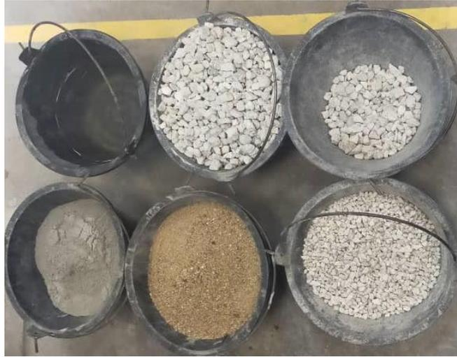
Figure 3.12: Raw Materials Preparation after Weighing Machine.
