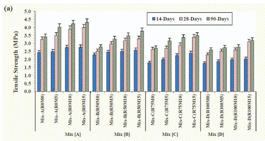
Figure 2.11: The Tensile Strength of Concrete with different Portion of Metakaolin used (Elhadi et al., 2023).
