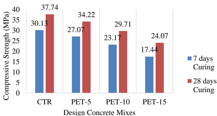
Figure 4.10: Compressive Strength of Various Design Concrete Mixes.
