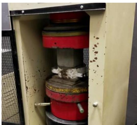
Figure 3.18: Compression Test of Cubic Specimen.
