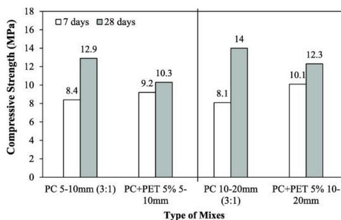
Figure 2.9: Compressive Strength of Concrete Mix with 5 % PET Content (Supit and Priyono, 2022).
