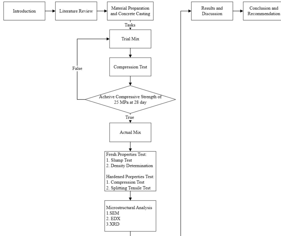
Figure 3.1: Flow Chart of Overall Work and Lab Experiment Procedure Detail.
