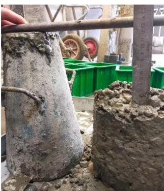
Figure 3.17: Slump Values of Fresh Concrete.
