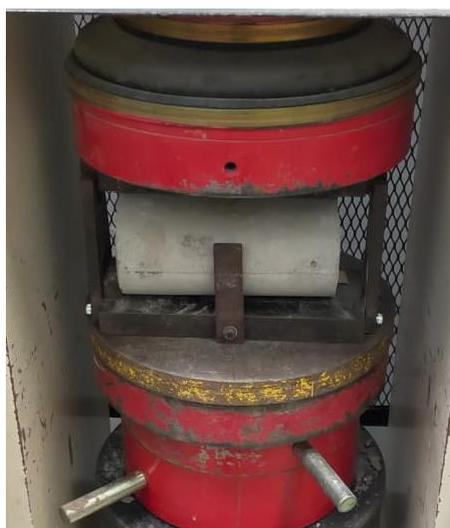
Figure 3.19: Splitting Tensile Test of Cylindrical Specimen.
