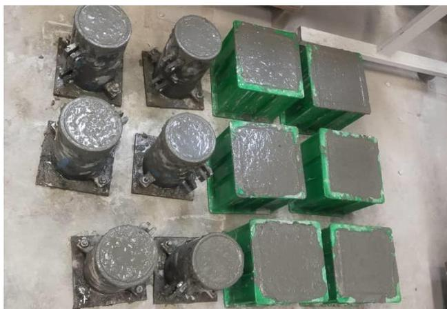
Figure 3.14: Hardening and Settling of Concrete Mix.
