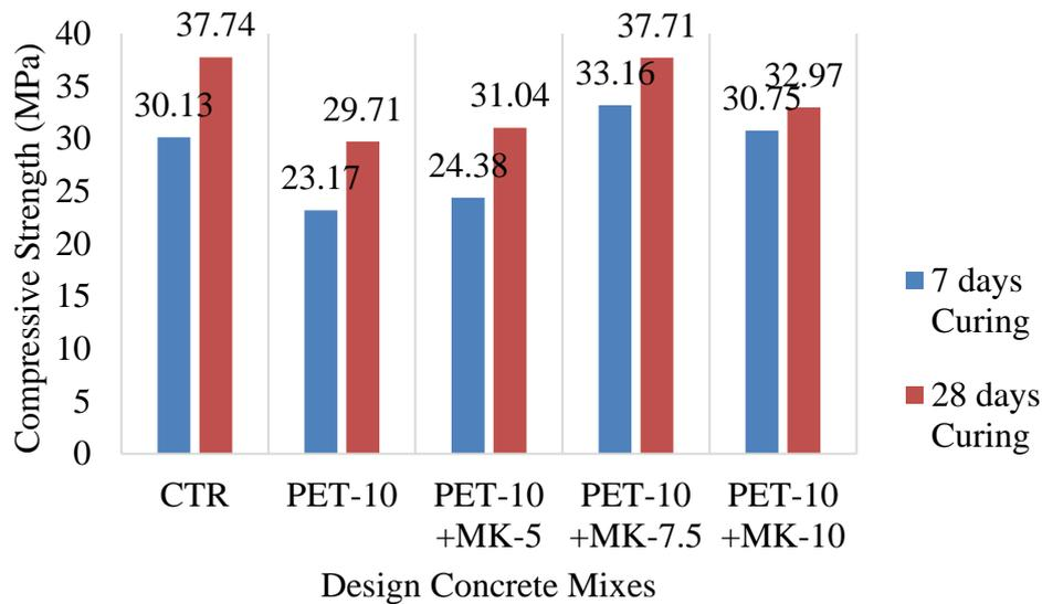
Figure 4.14: Compressive Strength of Various MK Content in PET-10.
