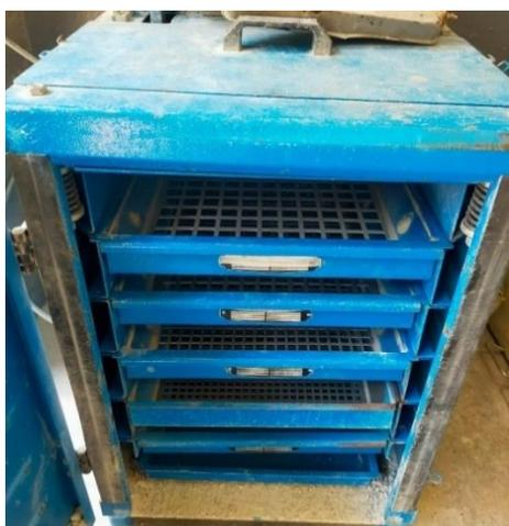
Figure 3.11: Machine for Coarse Aggregates Sieve Analysis.
