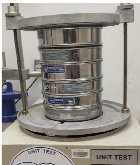
Figure 3.10: Machine for Fine Aggregates Sieve Analysis.
