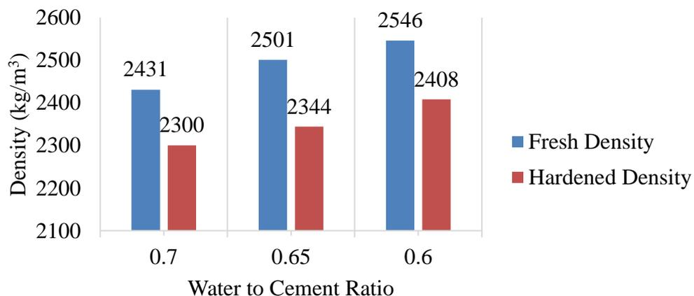
Figure 4.3: Fresh and Hardened Density of Trial Mixes of CTR.
