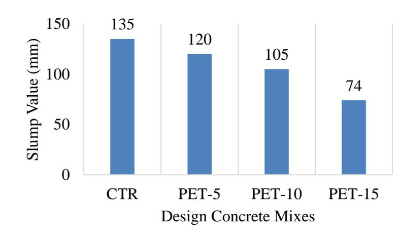
Figure 4.8: Slump Values of Various Concrete Mixes.
