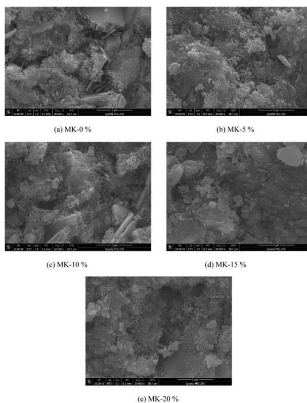
Figure 2.18: The Morphologies of Cement Paste with Different Metakaolin's Proportion (Li et al., 2022).
