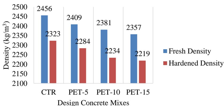
Figure 4.9: Fresh and Hardened Density of Various Concrete Mixes.
