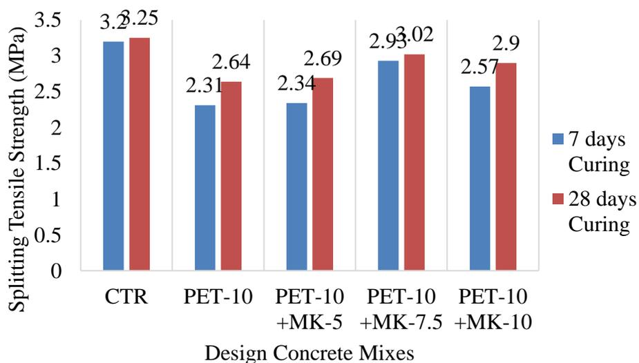
Figure 4.15: Splitting Tensile Strength of Various Design Concrete Mixes.
