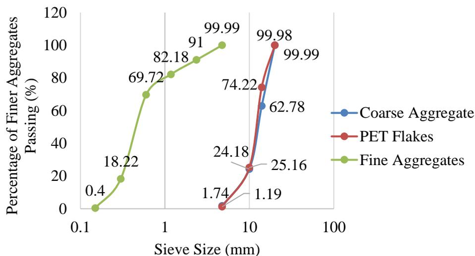
Figure 4.1: Distribution of Aggregates Particles Size.
