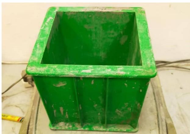
Figure 3.7: Cubic Mould.
