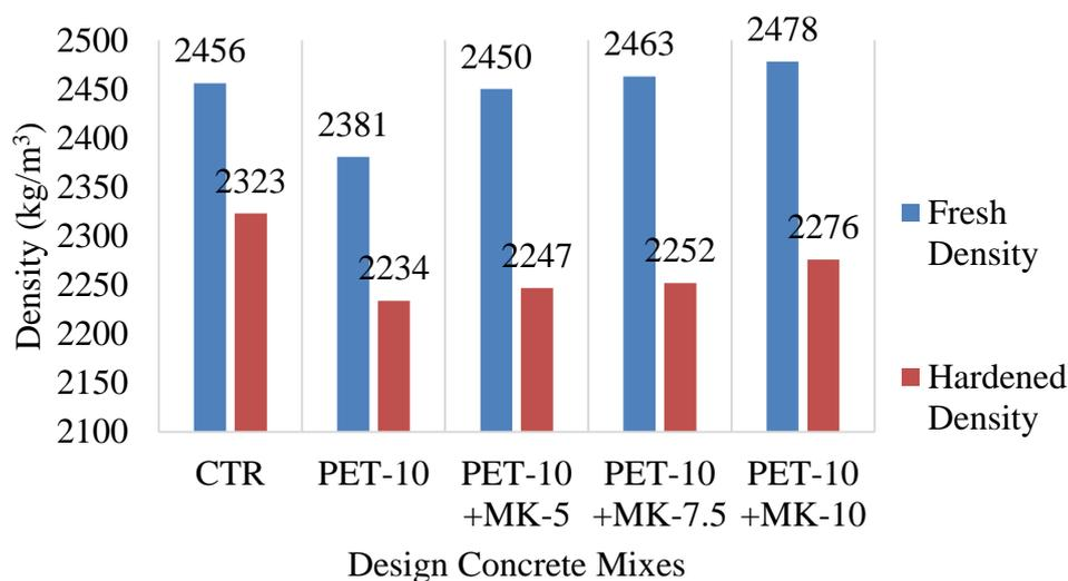
Figure 4.13: Fresh and Hardened Density of Various MK Content in PET-10.
