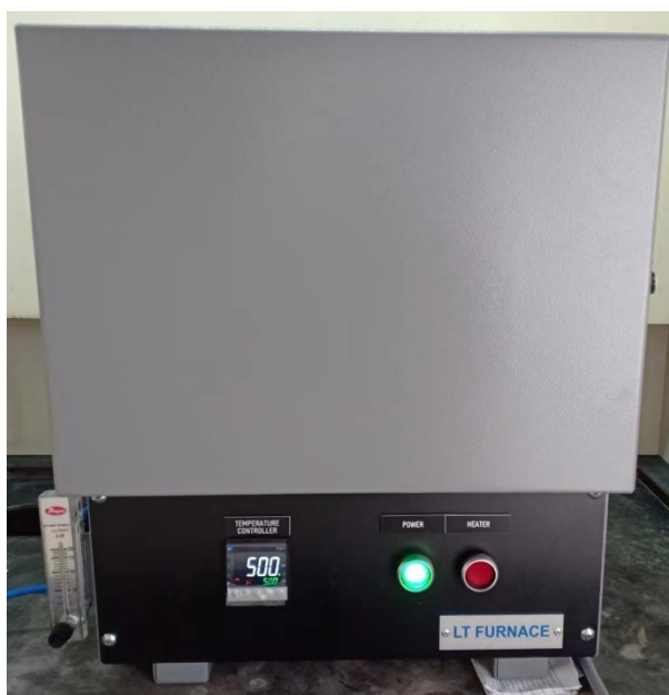
Figure I-2: Sulfation Roasting in Muffle Furnace.
