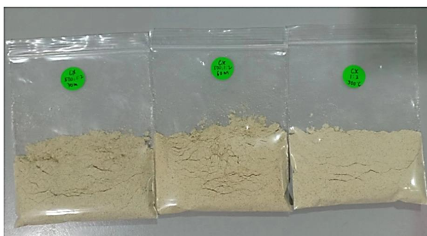
Figure I-6: Treated Coal Mining Sludge at Different Roasting Time.
