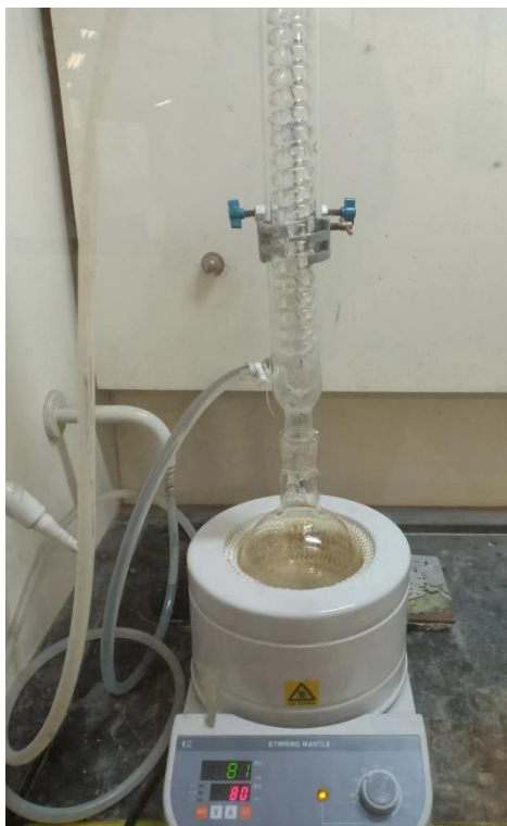
Figure I-3: Water Leaching with Heating Mantle Under Reflux.
