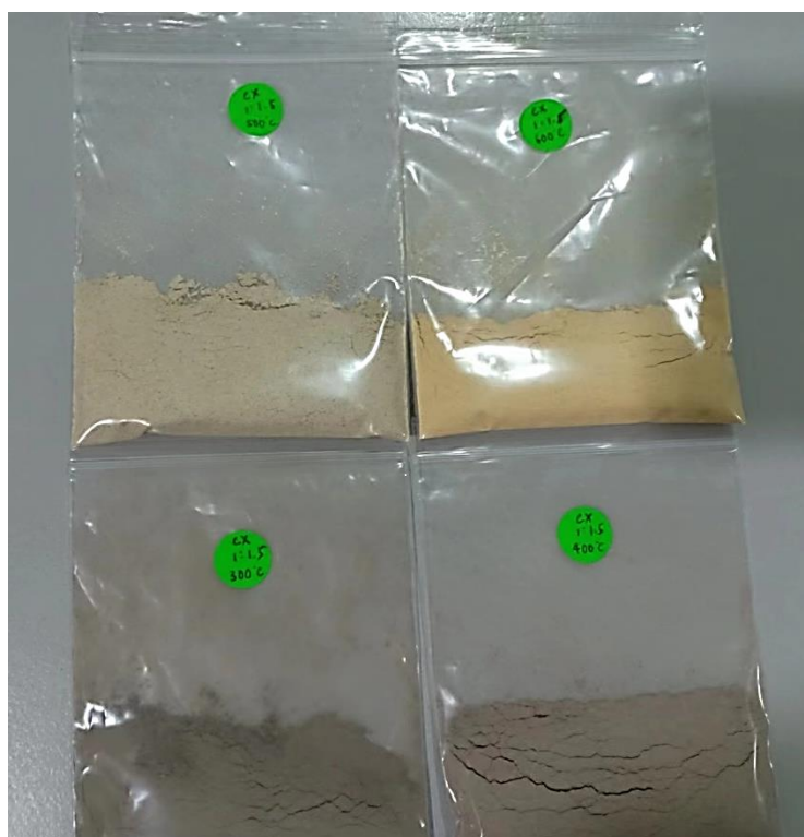
Figure I-4: Treated Coal Mining Sludge at Different Roasting Temperature.
