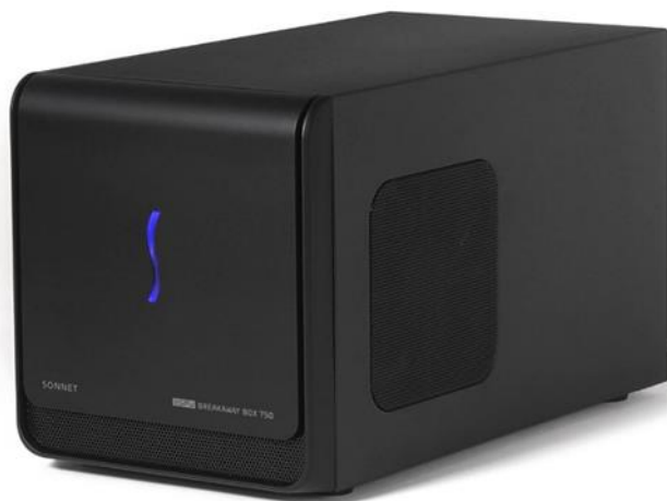
Figure 3.2: Sonnet eGPU Breakaway Box 750
