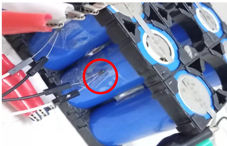
Figure 3.10: Thermistor taped to the battery body.
