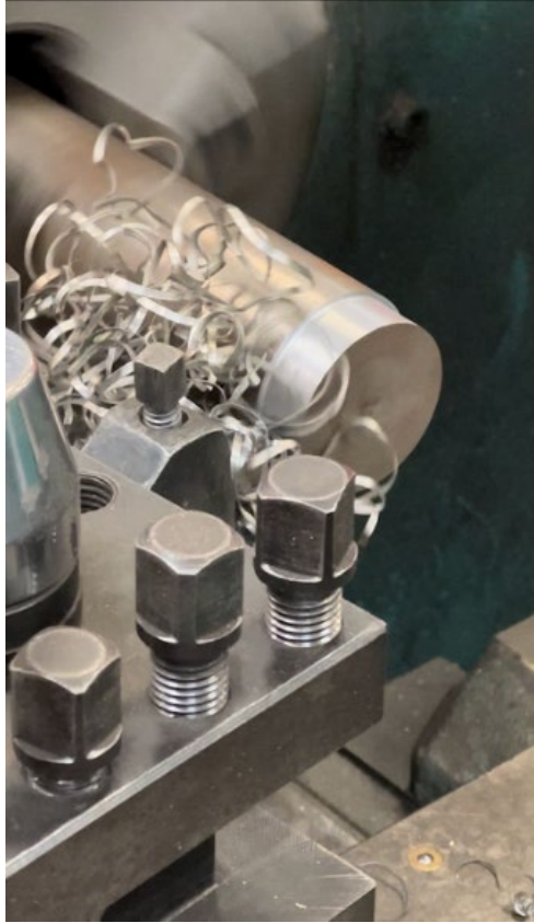
Figure 3.4: Lathe machine to obtain the required diameter of the metal cylinder
