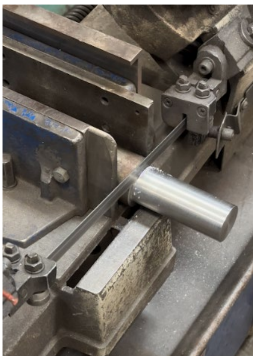
Figure 3.3: Bend saw to cut the metal bar
