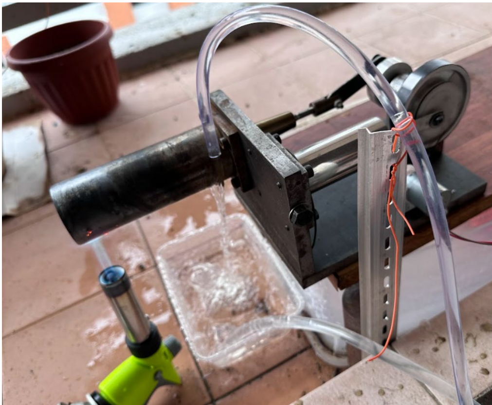
Figure 3.9: Cooling system attached to the Stirling engine
