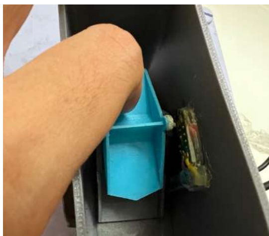
Figure 3.18: Image showing when the Hall Effect Sensor senses the magnet
