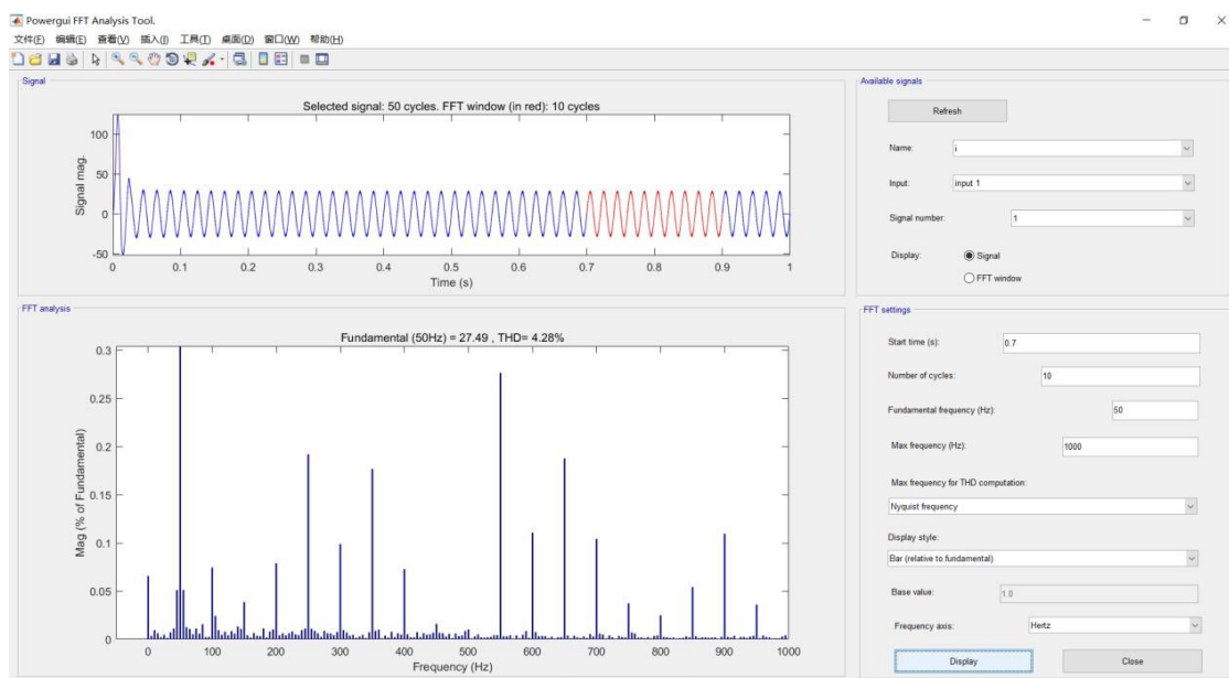
Figure 4.8 THD diagram of phase A
