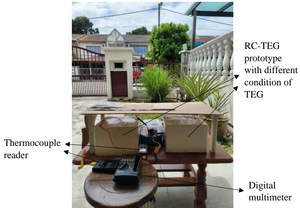
Figure 3.7: Experiment setup of RC-TEG
