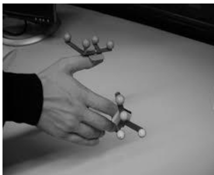
Figure 2.1 IRTTs mounted at user's fingers. Adapted from [5]
