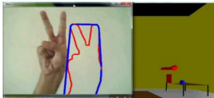
Figure 2.7 Gesture for moving up. Adapted from [6]
