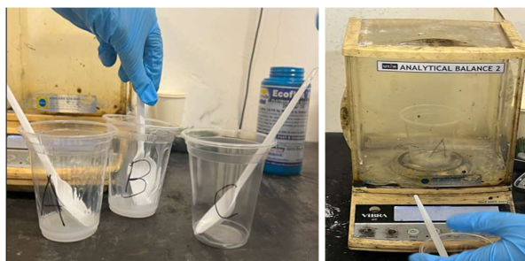
Figure 3.13: Preparation of Ecoflex.
