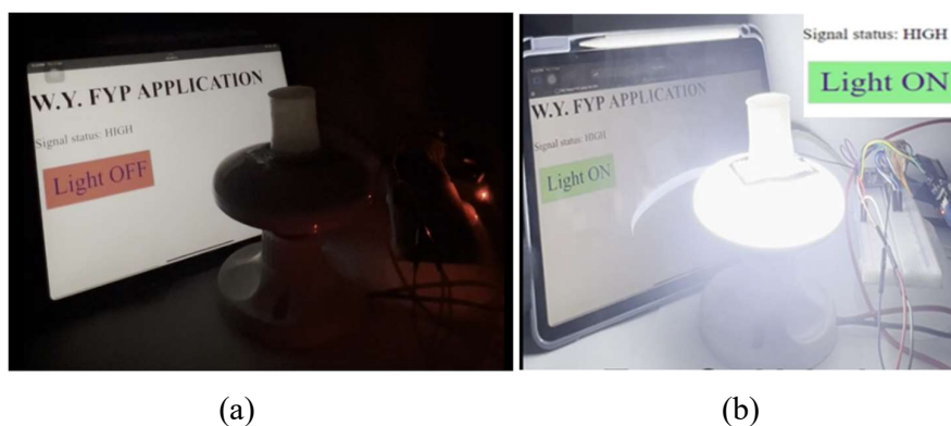
Figure 4.29: Light is (a) OFF and (b) Turned On with Ethyl Acetate DRA.
