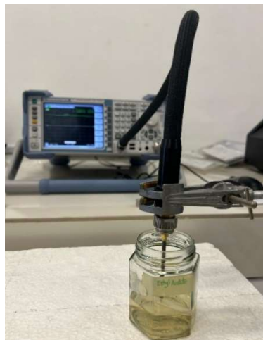
Figure 3.33: Setup of Liquid Dielectric Properties Measurement.
