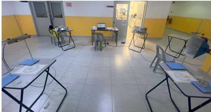
Figure 3.35: Setup of Far-field Measurement.
