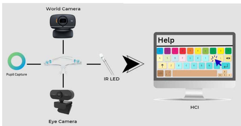
Figure 3.5: Overview of Head-mounted Eye Tracker Integrated with HCI
