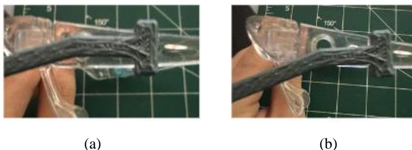
Figure 3.27: Placement of Female Extender: a) Initial Position Before Placement and b) Position After Placement
