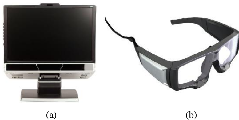
Figure 2.3: Types of Eye Trackers: (a) Screen-based Eye Tracker and (b) Head-mounted Eye Tracker (George, 2019)
