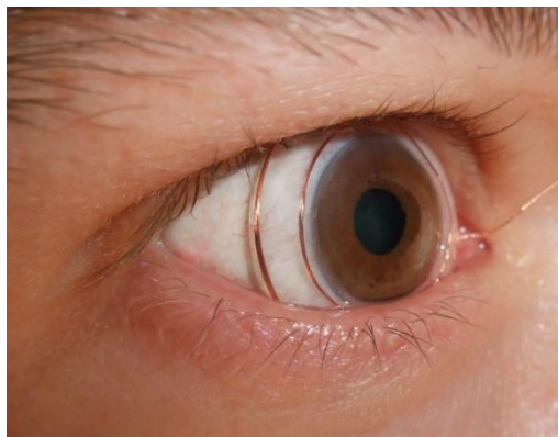
Figure 2.6: Scleral Search Coil Technique (Thankachan, 2018)
