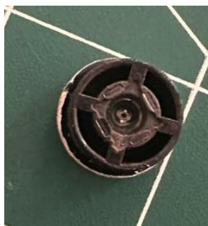
Figure 3.14: Camera Lens with Removed IR Filter
