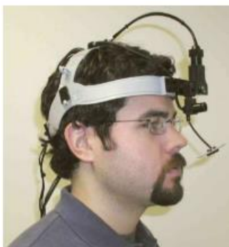
Figure 2.8: Video-based Head-mounted Eye Tracker (Alhamad et al. , 2022)
