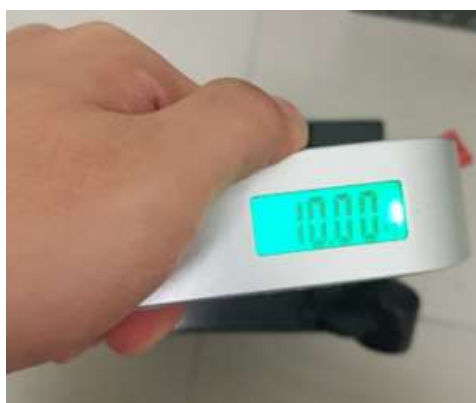
Figure 4.19: The Battery Weighs 10kg, as Displayed on the Weight Scale.
