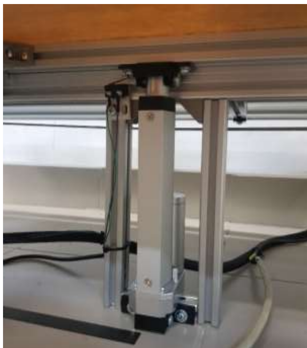
Figure 4.5: The 3D-Printed Brackets Are Mounted on the Electric Cylinder Linear Actuator.
