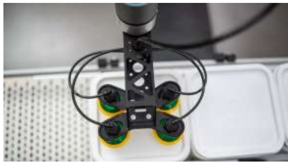
Figure 2.4: Vacuum Clamp Holding Item (Owen-Hill, 2023).
