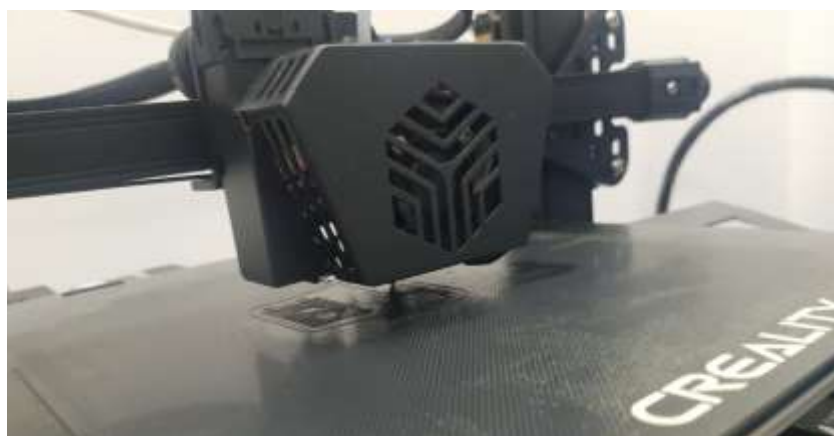
Figure 4.2: The 3D Printer Is Printing the Sensor Bracket.
