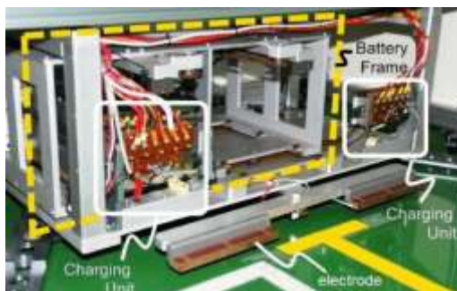
Figure 2.18: The Mechanical Structure of Two Charging Units Integrated Horizontally Linearly on Both Sides of the Carrier (Cheng Wu et al., 2009).
