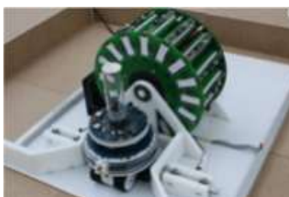
Figure 2.19: The Wheel-Shaped Charging Station with A Docked Marxbot (Vaussard et al., 2013).
