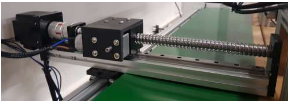
Figure 4.9: The Actuator Is Placed Horizontally on the Gantry Plate.
