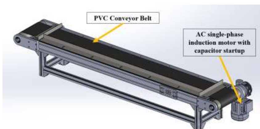
Figure 3.2: Conceptual Design of Bi-Directional Belt Conveyor.
