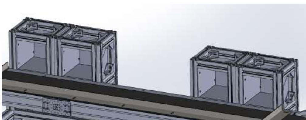
Figure 3.6: Two Independent Battery Storage Compartments on Each Side.
