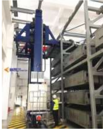
Figure 2.11: Yangshan Port Battery Replacement Station for Heavy Truck (Jasmine Lihua & Danilovic, 2021).
