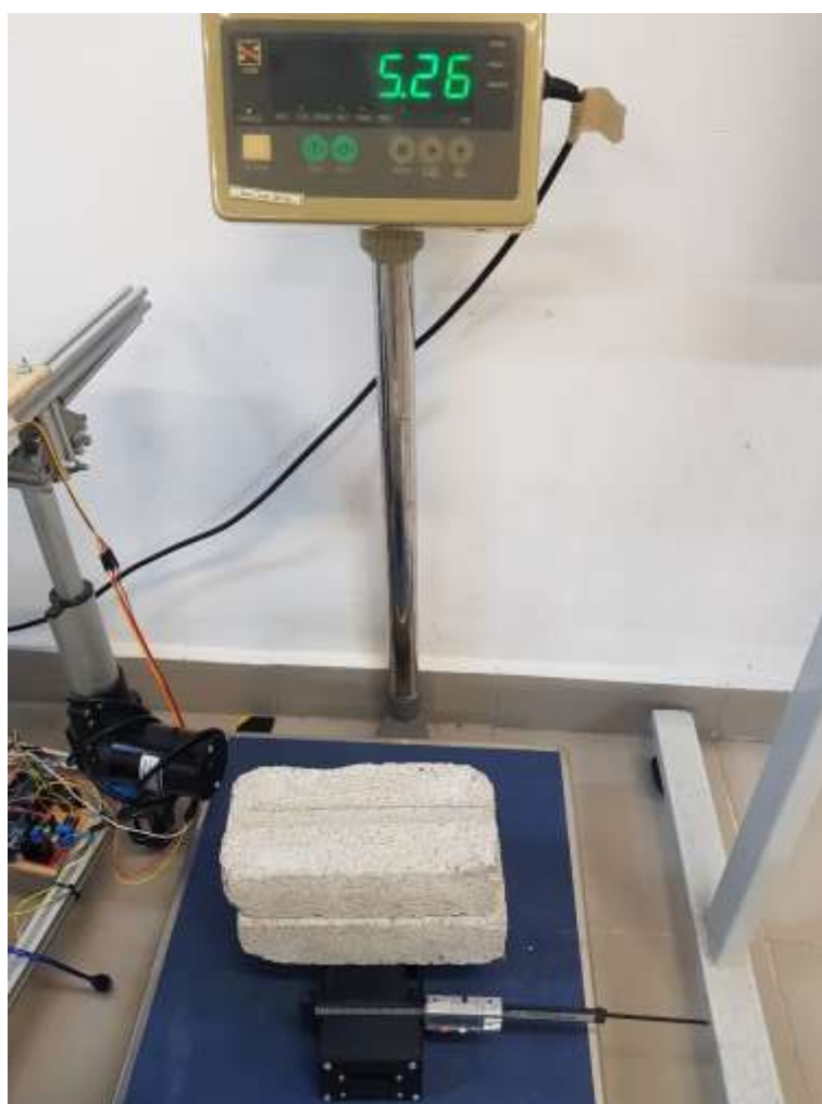
Figure 4.28: The Setup of the Stress Test.
