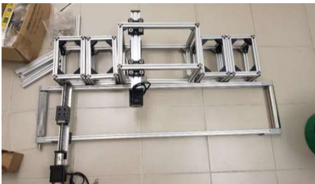
Figure 4.3: The Main Structure Is Constructed Using Aluminium Profiles.
