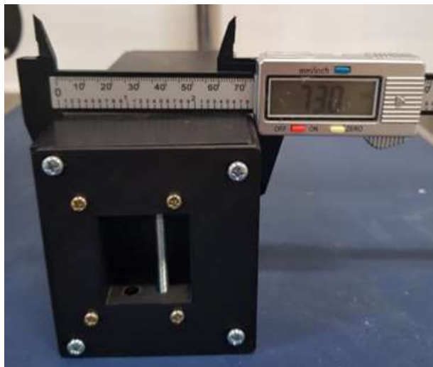
Figure 4.30: The Dimensions of the Battery Enclosure Side Before the Experiment.
