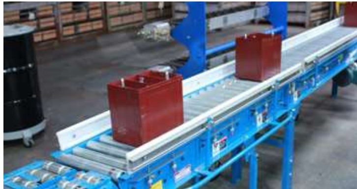
Figure 2.14: The Battery Is Being Transported on a Powered Roller Conveyor (condrives, 2013).
