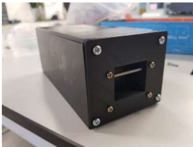
Figure 4.18: The Battery Module Has Been Assembled.
