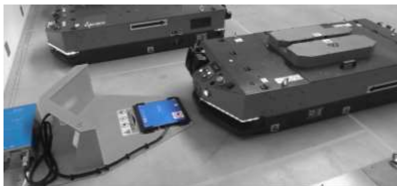
Figure 2.24: Wireless Charging of AGVs Using Wiferion Technology (Edwards, 2021).
