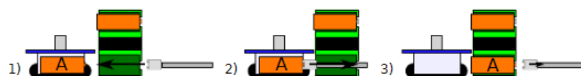
Figure 2.3: The Mechanical Structure of A Linear Motion with Tightenable Gripper (Vaussard et al., 2013).
