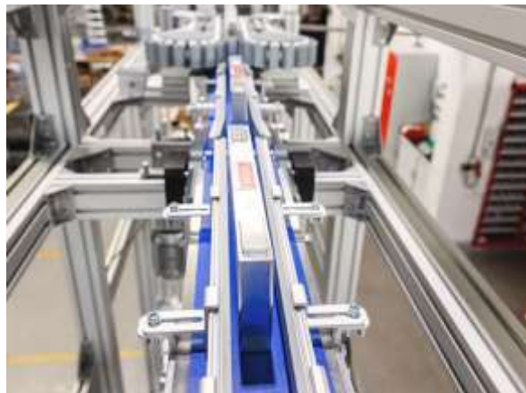
Figure 2.13: The Battery is Being Transported on a Belt Conveyor (FLEXLIN K, 2021).
