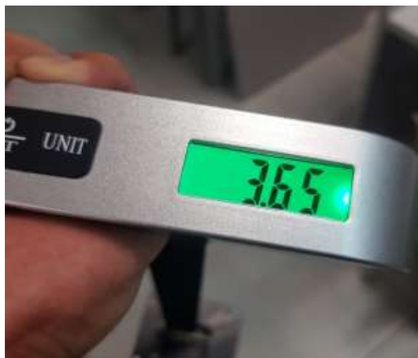
Figure 4.35: The Handle of The Battery Undergoes a Test With A Load Of 3.65 Kilograms.
