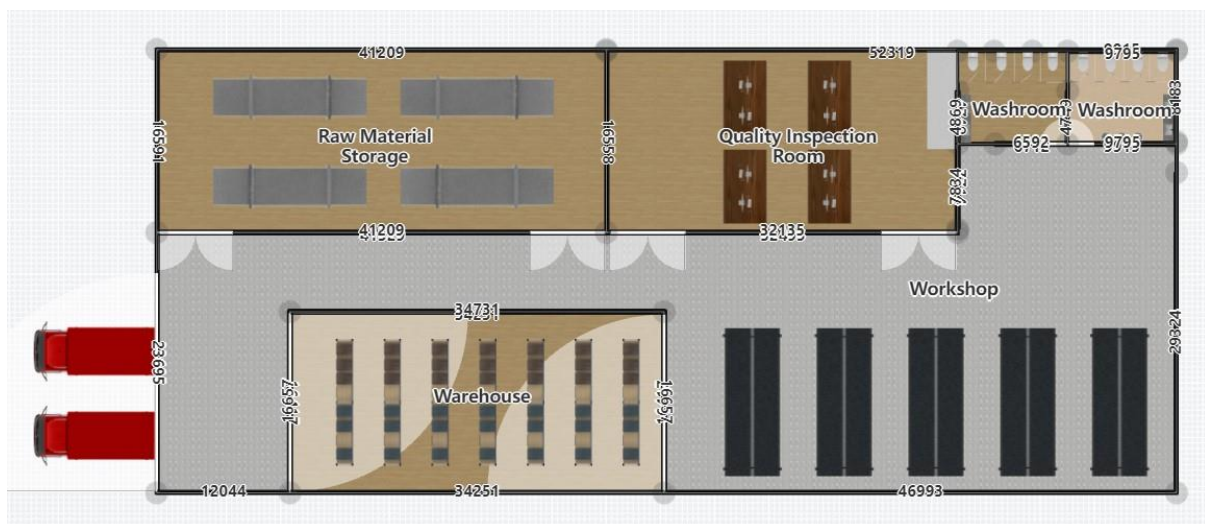
Figure 5.5: Ground Floor: Manufacturing Plant Design
