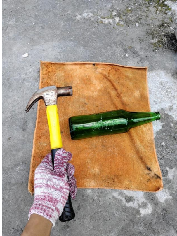
Figure 3.4: Hammering process for glass waste bottle.
