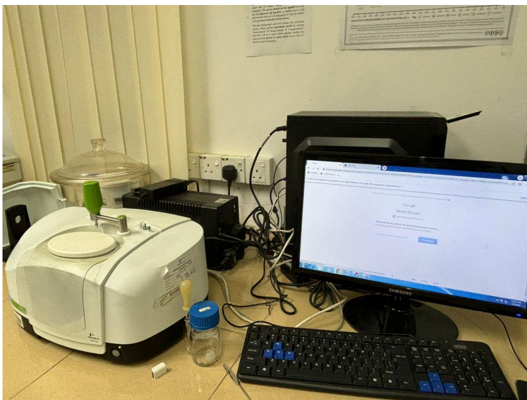
Figure 3.14: Attenuated Total Reflectance Fourier Transform Infrared (ATR-FTIR) spectroscopy.
