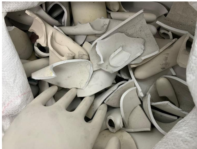
Figure 3.6: Glove Former waste from Kitaran Recovery Sdn. Bhd.
