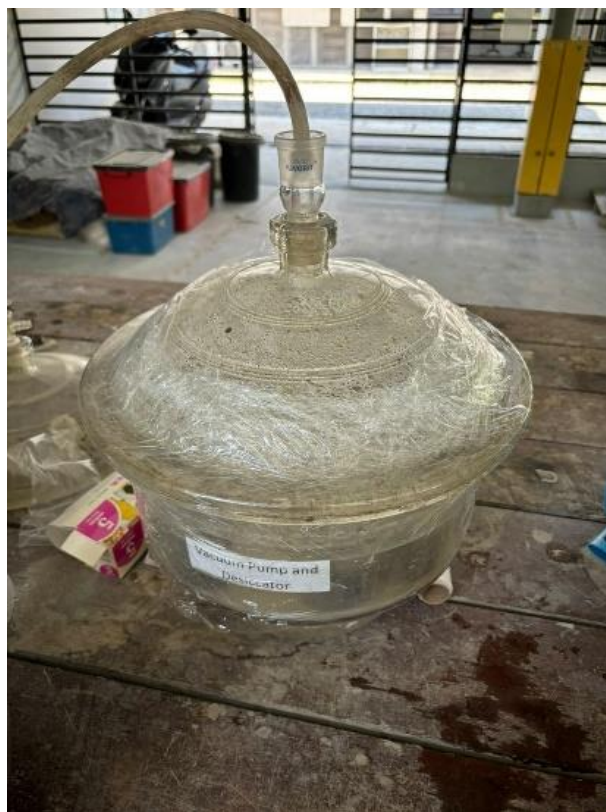
Figure 3.18: Vacuuming Process for Geopolymer
