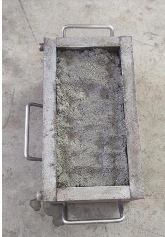
Figure 3.6: CSB Steel Mould.
