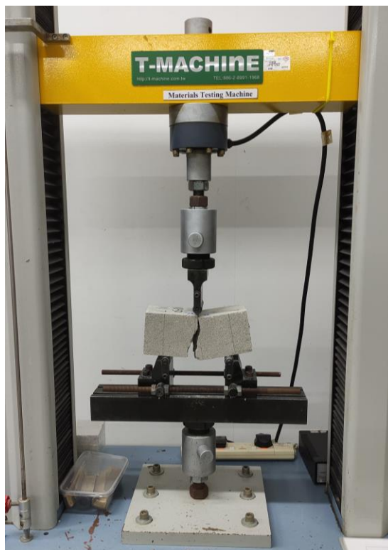
Figure 3.12: Flexural Strength Test.
