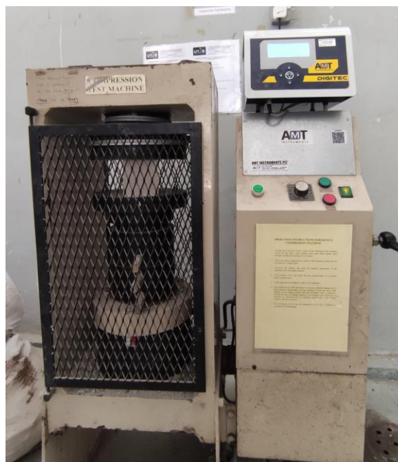
Figure 3.11: Compressive Strength Test.
