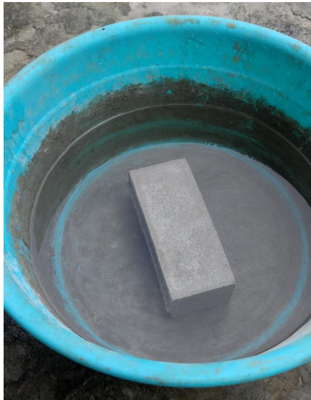
Figure 3.14: Water Absorption Test.
