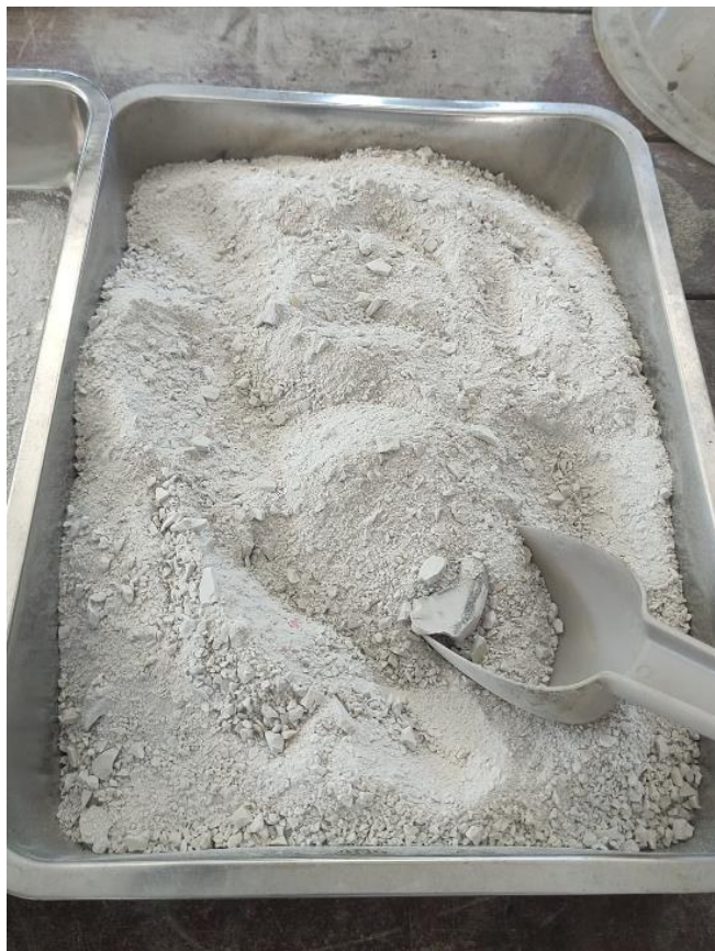
Figure 3.4: Glove Former Waste.
