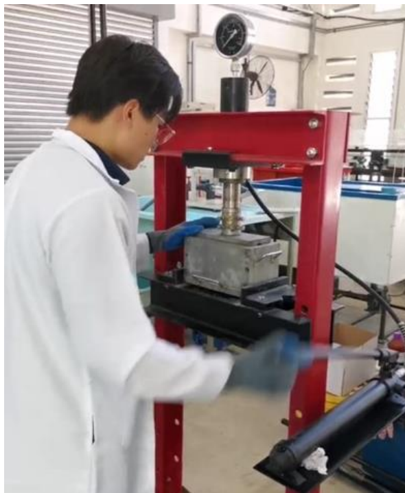
Figure 3.7: Compaction of CSB with Hydraulic Shop Press.
