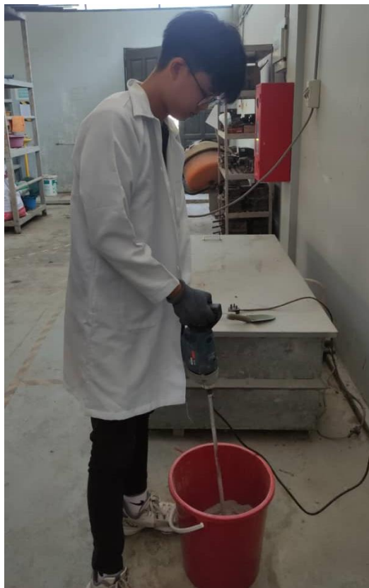
Figure 3.6: Mixing Process of CSB Specimens.
