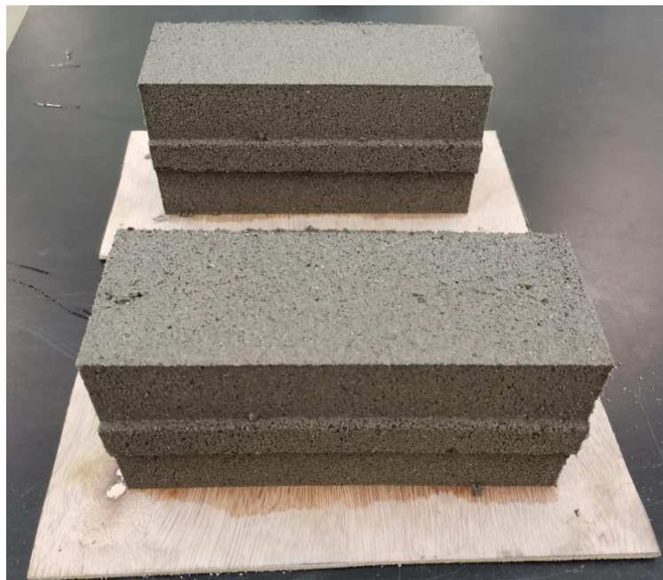
Figure 3.9: CSB Specimens after Demoulding.
