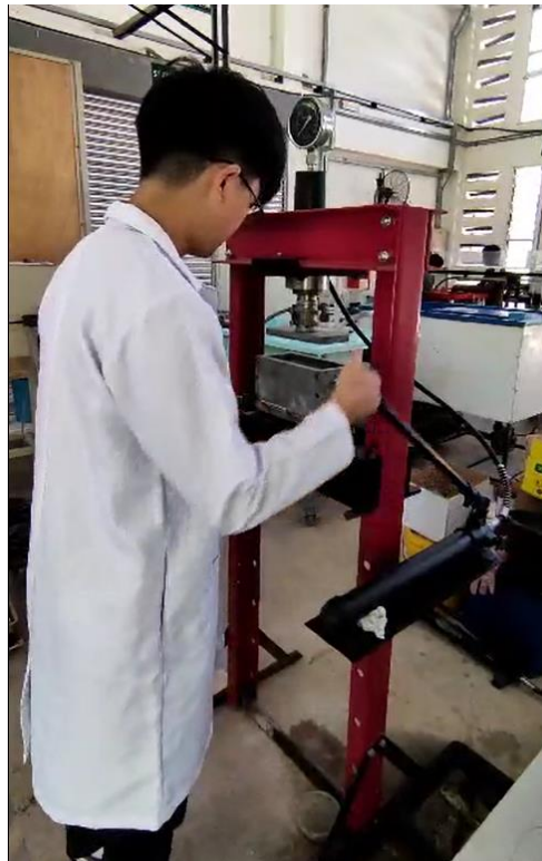
Figure 3.8: Compression of Specimens using Hydraulic Shop Press.
