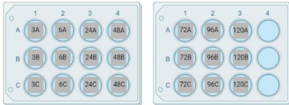
Figure 3.3: Test coupons arrangement in 12 wells culture plate and its labelling based on the incubation time (3 h, 6 h, 24 h, 48 h, 72 h, 96 h and 120 h) and replicated in thrice.
