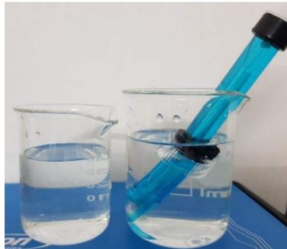
Figure 5.12: pH 4.01 and pH 7.00 Buffer Solution with pH Probe immersed
