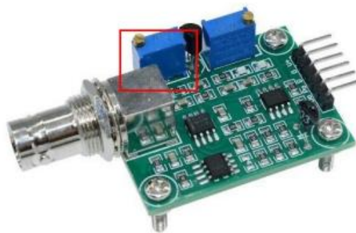
Figure 5.9: Highlighted area on reference electrode is Potentiometer
