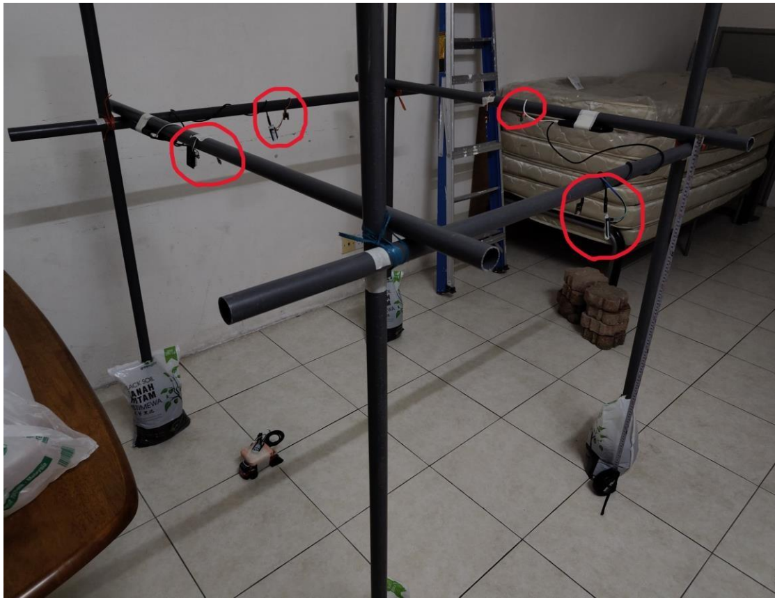
Figure 5.4 Indoor Positioning System Setup
