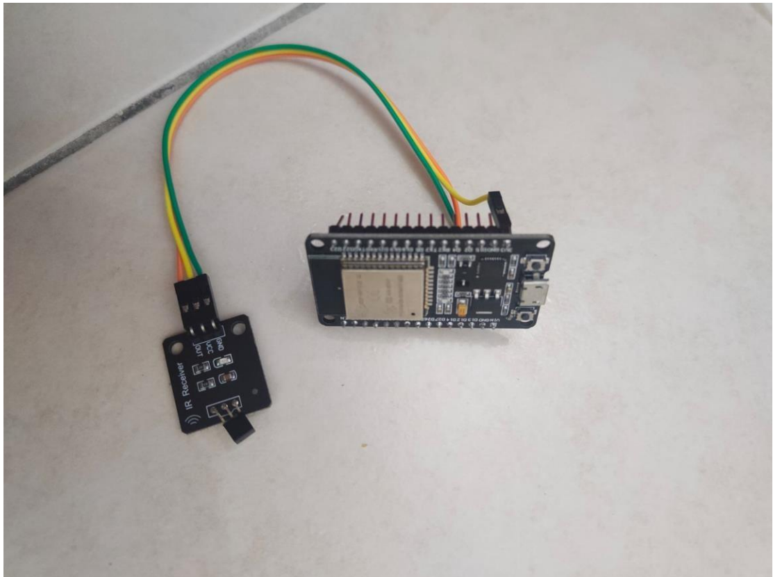
Figure 5.2 Connection between Infrared Receiver with ESP32 Development Board
