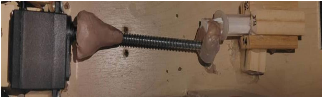
Figure 5.1 Modification of servo motor into hydraulic actuator
