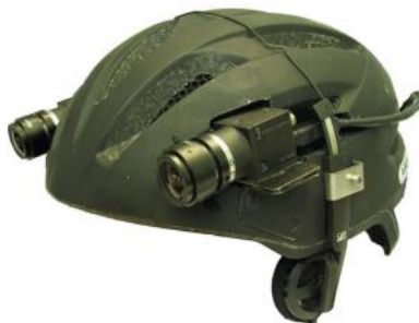
Figure 2.1.1 Hardware configuration of a bicycle helmet, binocular camera, and earphones [2]
