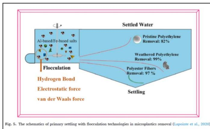
**Figure 2.6.4:** The primary settling with flocculation process (Lapointe et al., 2020).
