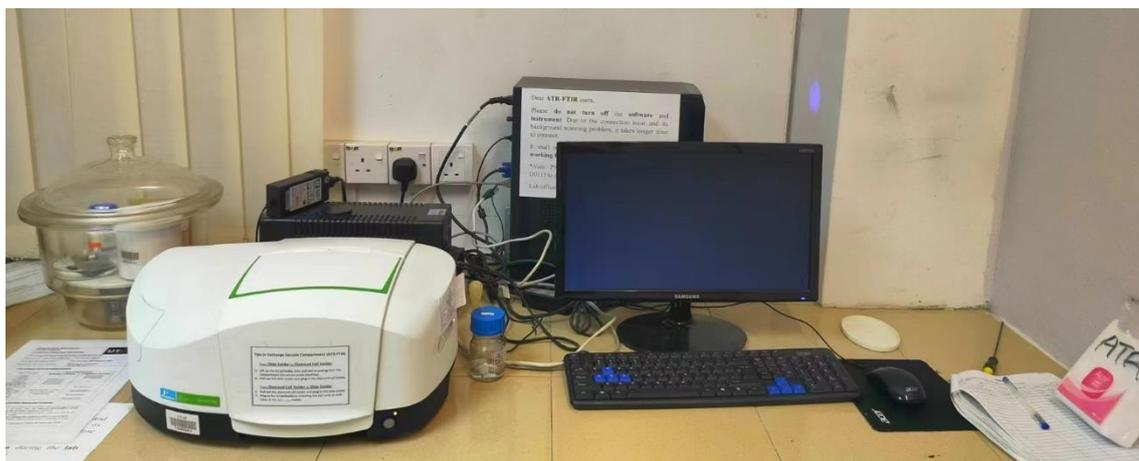
**Figure 3.9:** PerkinElmer Spectrum Two FTIR- ATR Spectrometer
