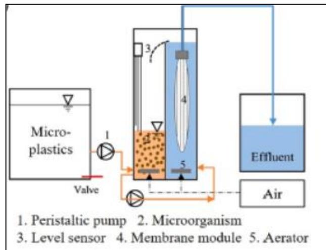
**Figure 2.6.6:** MBR system (Li et al., 2020)
