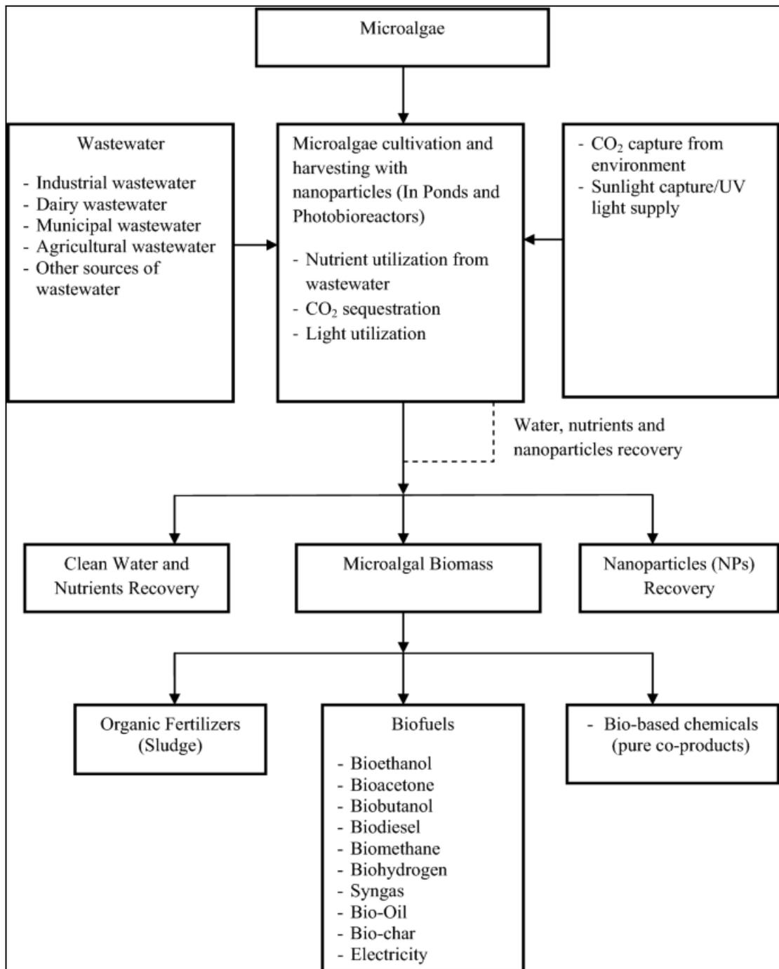
**Figure 2.9.4:** Flow diagram of processing microalgae for general uses through harvesting of microalgal biomass (Hossain, Mahlia and Saidur, 2019).
