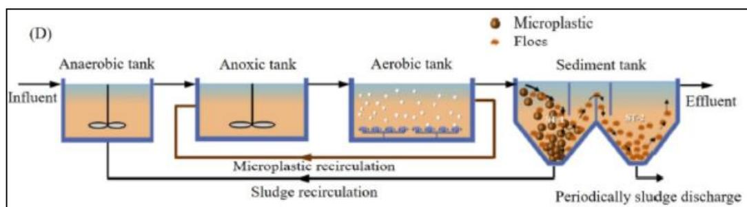
**Figure 2.6.8:** Process of A<sup>2</sup>O system (Liu et al., 2020)
