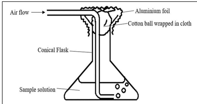
**Figure 3.5.1:** Setup of microalgae and microplastic coexistence in Block J.
