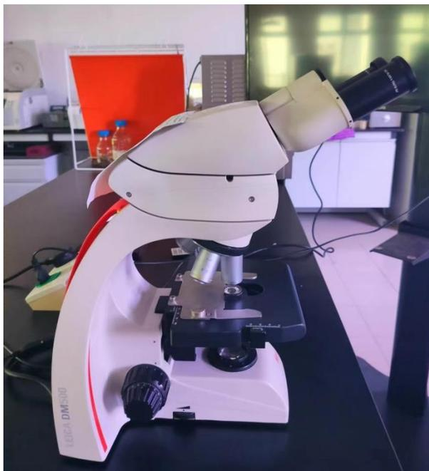
**Figure 3.8:** Leica DM500 microscope
