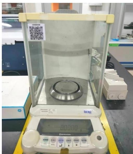
**Figure 3.7.3:** Shimadzu AUX320 Analytical Balance
