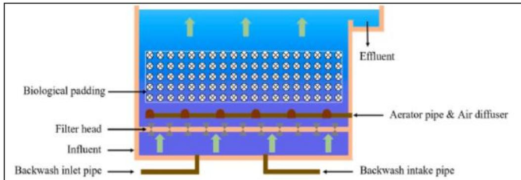
**Figure 2.6.7:** Process of biofilter system (Liu et al., 2020)
