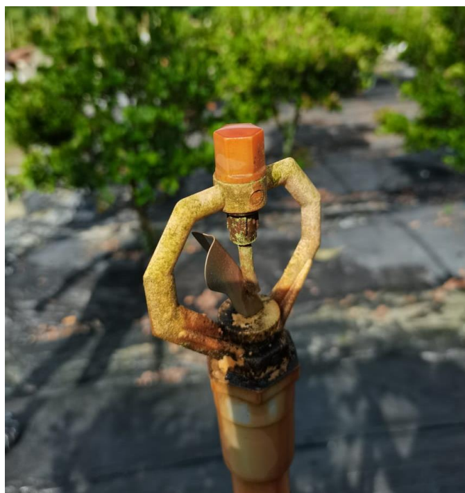
Figure A9: Iron Staining and Clogging of Irrigation System in Miracle Berry Farm
