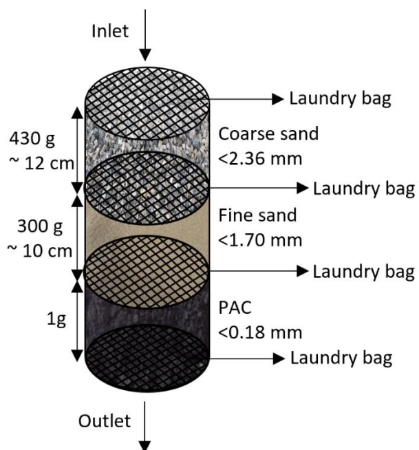
Figure 3.4: Filter System Arrangement with PAC
