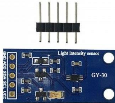
Figure 3.3. BH1750 digital light intensity sensor module.
