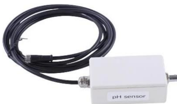
Figure 3.5: pH sensor in TPY series V13.0.1 (Nanbeinstrument, China).
