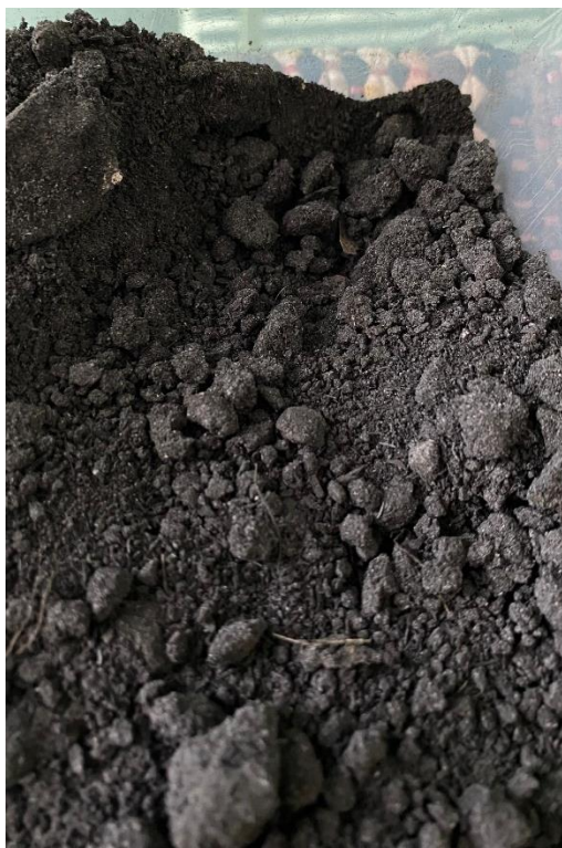
Figure 4.5: Palm Oil fuel ash from Air Kuning palm oil factory.
