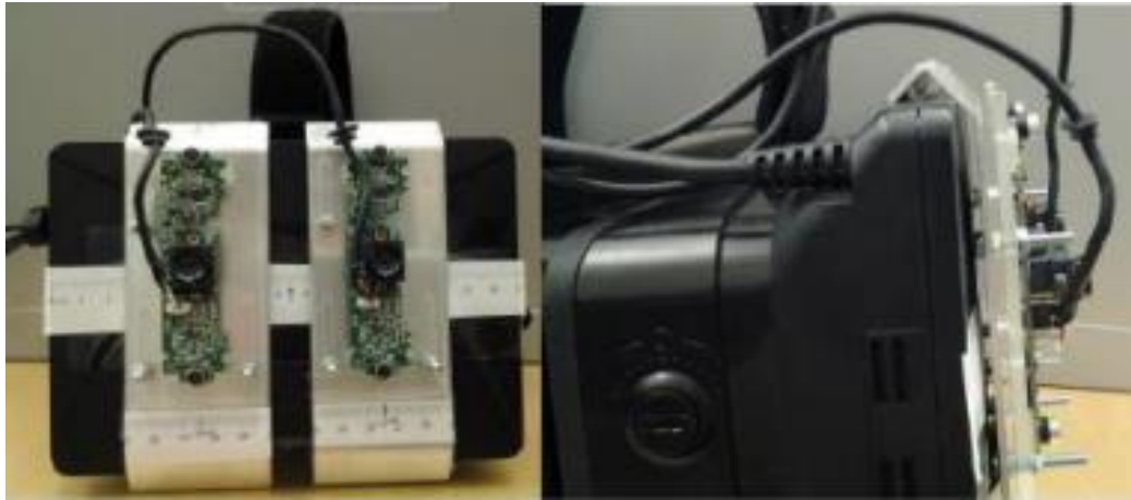
Figure 2. 8: Oculus rift prototype with cameras attached to front.
