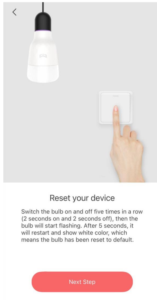
Figure 5. 11: Image describes how to reset the light bulb
