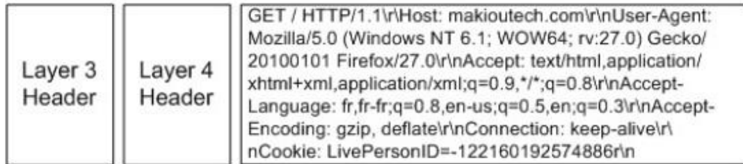
Figure 2.6: The header of the raw HTTP request packet [25].
