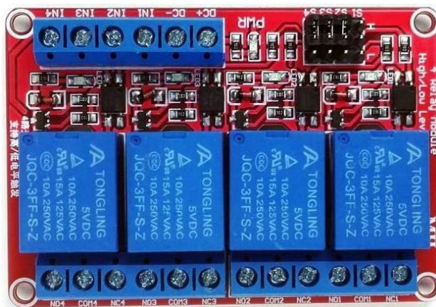
Figure 3.7: 4-Channel 5V Relay (Keim, 2024).
