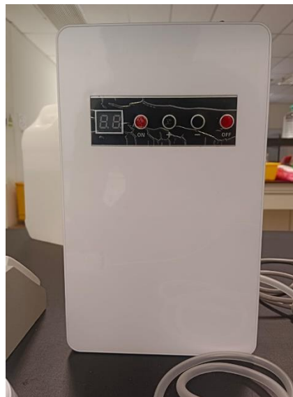
Figure 3.5: Ozone Generator Used in N012 Lab.
