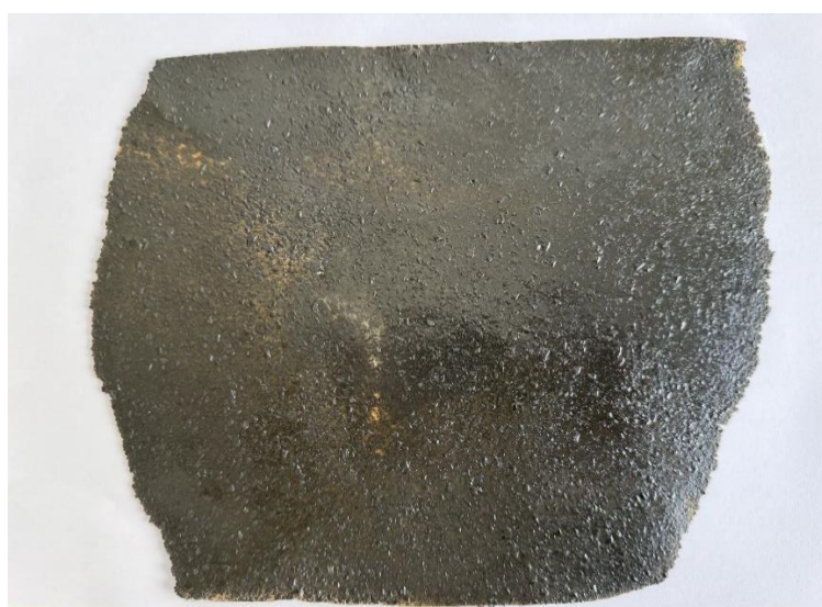
Figure 3.5: Sample of PVC/rNBR after going through hot and cold press.
