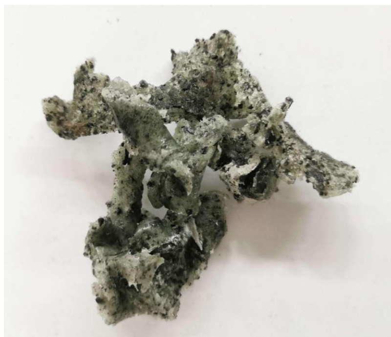
Figure 3.3: Sample of plasticized PVC/rNBR after melt blending.
