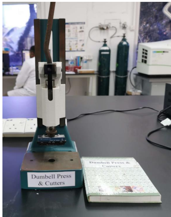
Figure 3.7: Dumbbell press and cutter and dumbbell shape samples.
