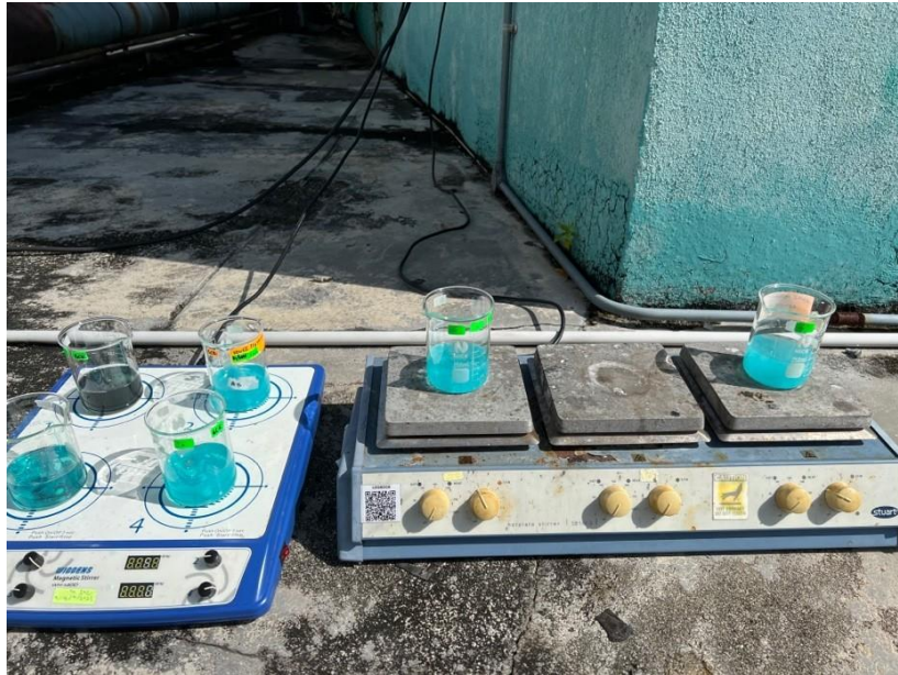
Figure 3.9: Experiment Setup for photodegradation of Malachite Green dye in greywater.
