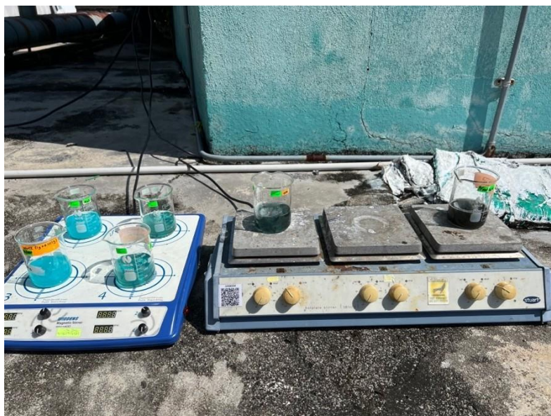
Figure 3.7: Experiment Setup for photodegradation of Malachite Green dye in distilled water.
