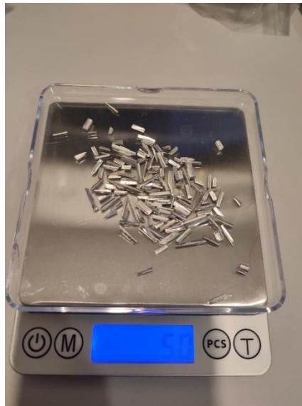
Figure 3.11: Measuring the aluminium scraps.
