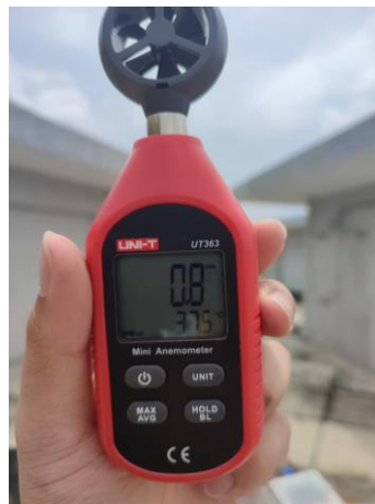
Figure 3.14: Measuring ambient temperature and wind speed using UNI-T UT363 Anemometers.
