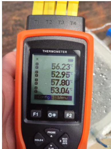
Figure 3.13: Measuring temperature using Yowexa YET-640X Thermometer.
