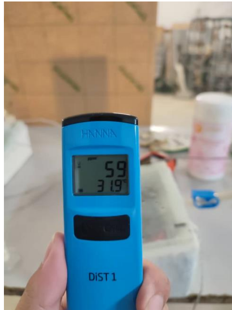
Figure 3.16: Measuring TDS using HANNA HI98301 TDS tester.
