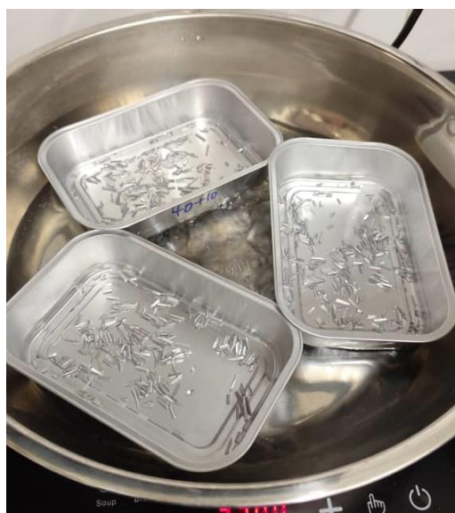
Figure 3.12: Hot water bath onto the basin to melt the paraffin wax.
