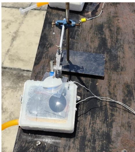
Figure 3.19: Prototype setup with Fresnel lens.
