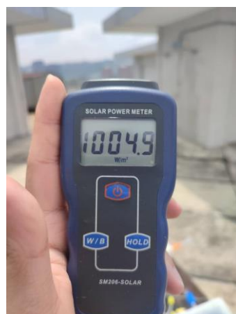
Figure 3.15: Measuring Solar Irradiance using SM206 Digital Solar Power Meter
