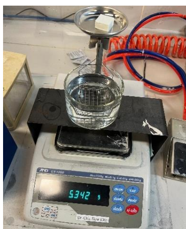
Figure 3.11: Apparatus setup for Archimedes' method.
