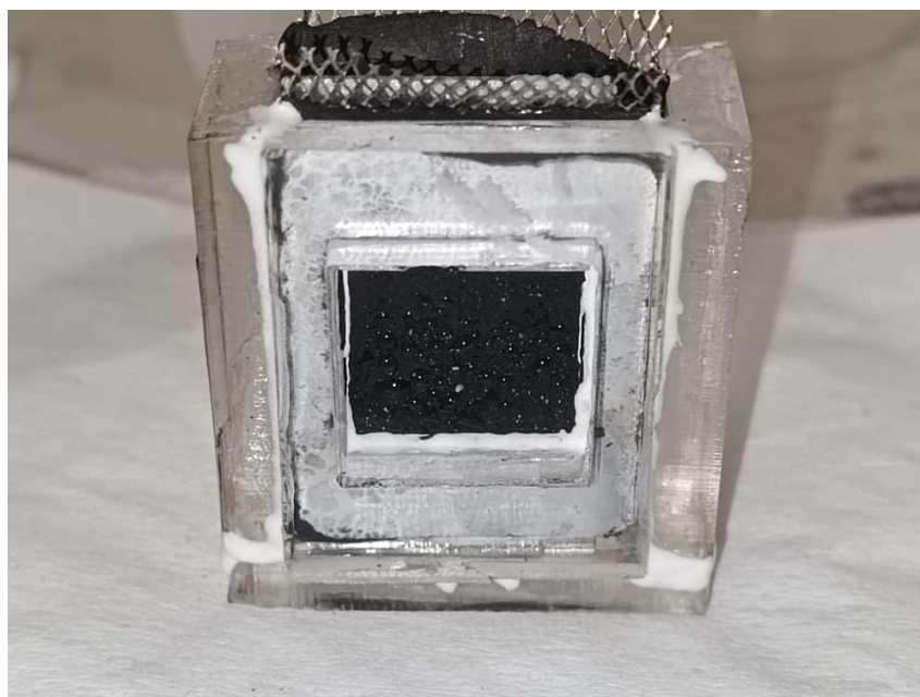
Figure 5.1: Water Leakage Found after Long Period of Operation
