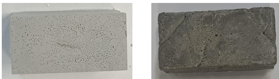
Figure 4.6: Surface finishing of cast product using (a) silicone mold; (b) 3D resin mold
