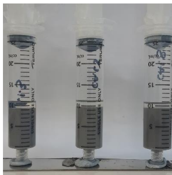
Appendix A-3: Set up of sediment test with different concentration of Acetone
