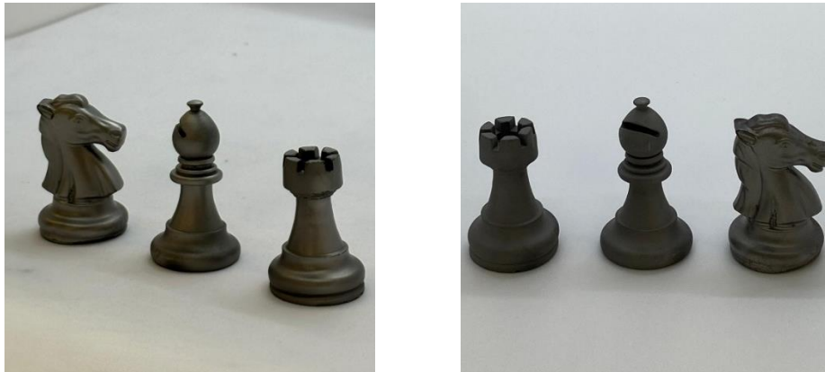
Appendix A-1: Cast products of sintered part and green part.
