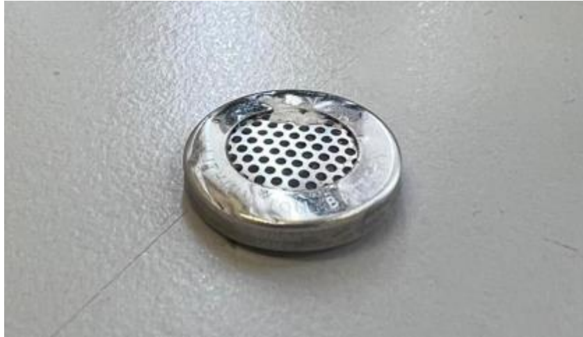
Figure 3.2: Overall design of aluminium-air battery.
