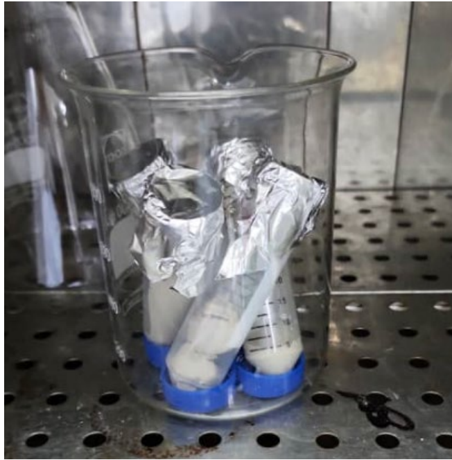
Appendix M: Oven is used to dry the kaolin precipitate.
