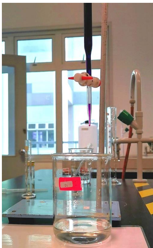
Figure 3.6: Redox Titration with Standard KMnO 4 solution
