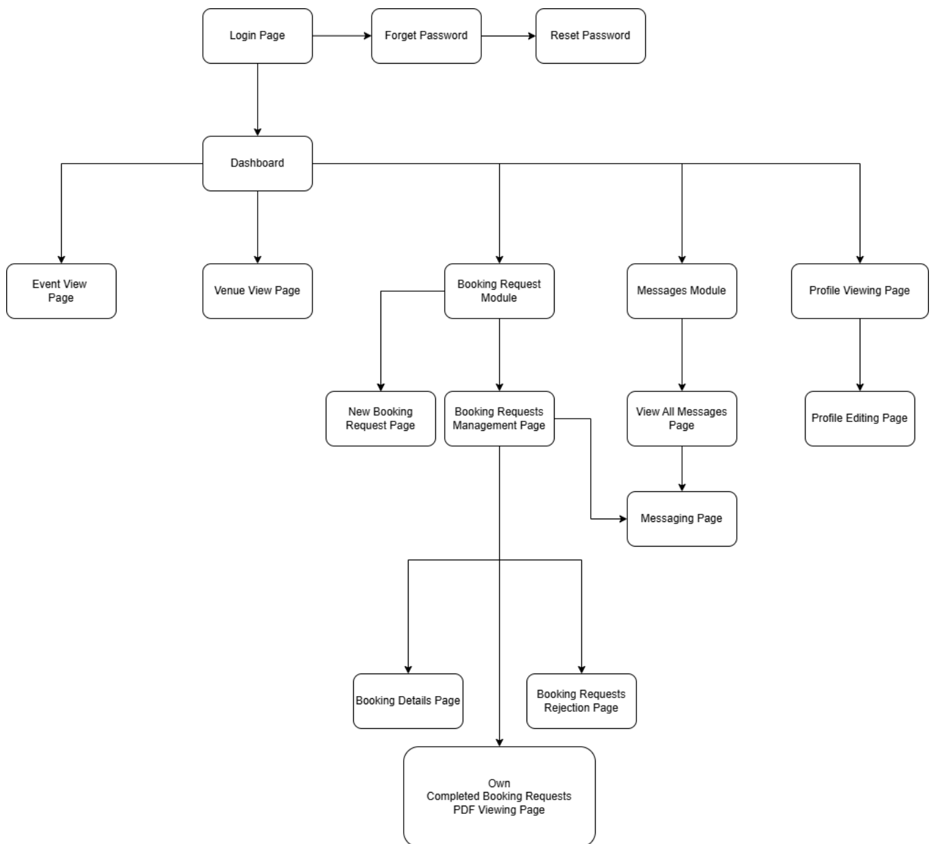
Figure 4.10: Interface Flow Diagram for the non-admin users in the UTAR Venue/Classroom Booking Web Portal
