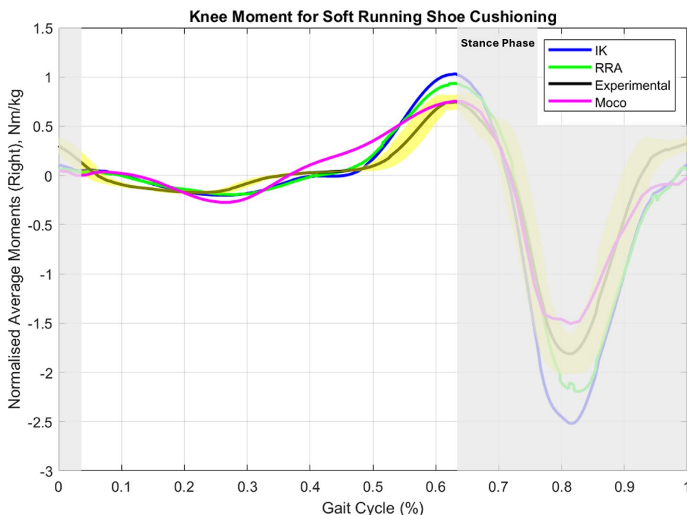
Figure 4.4: Knee Moment Gait for Soft Running Shoe Cushioning
