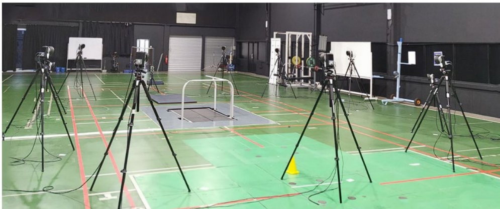
Figure 3.2: The Cameras Setup of the Motion Capture System (Boon, 2023)
