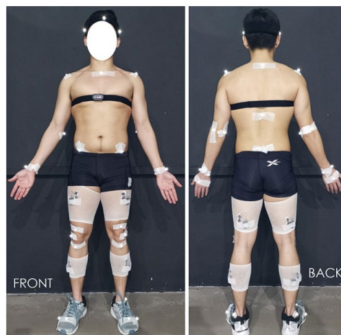
Figure 3.3: The Qualisys Optical Markers Position of Placements (Boon et al., 2022)
