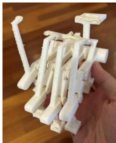
Figure 4.10: Broken Frames of the Conceptualised 4 Fingers Part.
