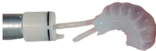
Figure 4.2: Deformation of the soft actuator.
