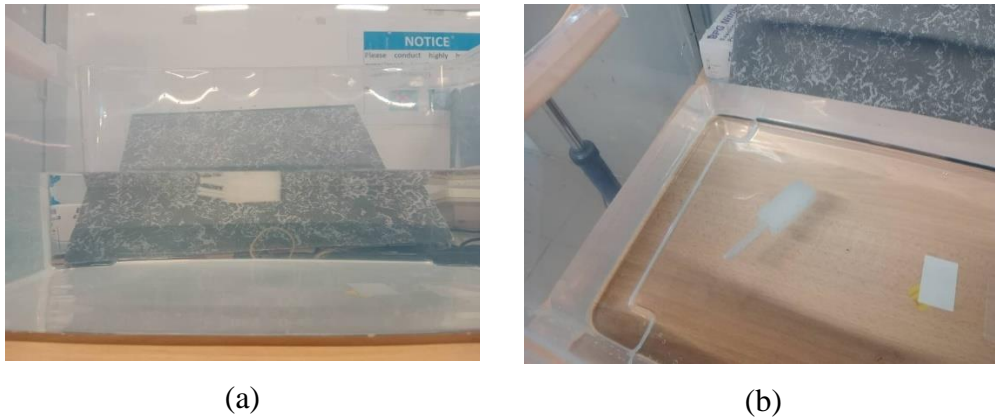
Figure 3.16: Soft actuator floating on water surface from (a) side view and (b) isometric view.
