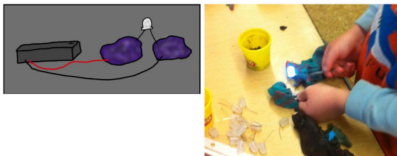
Figure 2.12: Simple circuit conductive dough with LED. Reprinted with permission from copyright 2018 Springer Nature.
