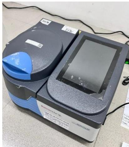
Figure 3.6: Thermo Fisher Scientific Genesys 180 model of UV-Vis analysis.
