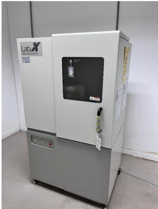
Figure 3.8: Shimadzu XRD 6000 model for XRD analysis.
