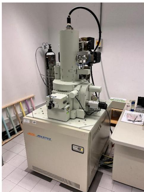
Figure 3.7: JSM-6701F and Oxford Instruments X-Max 50mm<sup>2</sup> models of SEM-EDX analysis.
